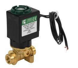
Spartan solenoid valve, 2-way, 2-position, N.C., low lead brass body, 1/8in female NPT inlet(s), 1/8in female NPT outlet(s), Cv=0.61, 80 psi maximum operating pressure, 120 VAC operating voltage, 18in 22 AWG pigtail.
