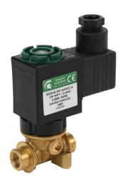
Spartan solenoid valve, 2-way, 2-position, N.C., low lead brass body, 1/8in female NPT inlet(s), 1/8in female NPT outlet(s), Cv=0.61, 60 psi maximum operating pressure, 24 VDC operating voltage, 18mm DIN style wiring plug.
