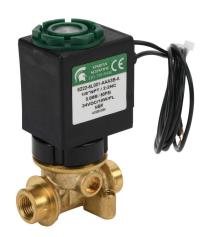
Spartan solenoid valve, 2-way, 2-position, N.C., low lead brass body, 1/8in female NPT inlet(s), 1/8in female NPT outlet(s), Cv=0.61, 60 psi maximum operating pressure, 24 VDC operating voltage, 18in 22 AWG pigtail.
