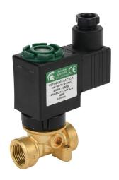
Spartan solenoid valve, 2-way, 2-position, N.C., low lead brass body, 3/8in female NPT inlet(s), 3/8in female NPT outlet(s), Cv=0.52, 125 psi maximum operating pressure, 120 VAC operating voltage, 18mm DIN style wiring plug.
