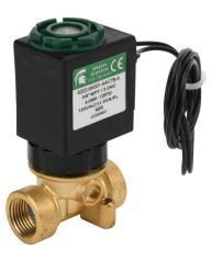
Spartan solenoid valve, 2-way, 2-position, N.C., low lead brass body, 3/8in female NPT inlet(s), 3/8in female NPT outlet(s), Cv=0.52, 125 psi maximum operating pressure, 120 VAC operating voltage, 18in 22 AWG pigtail.
