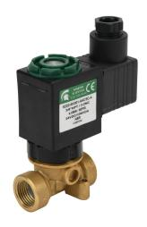
Spartan solenoid valve, 2-way, 2-position, N.C., low lead brass body, 3/8in female NPT inlet(s), 3/8in female NPT outlet(s), Cv=0.52, 90 psi maximum operating pressure, 24 VDC operating voltage, 18mm DIN style wiring plug.
