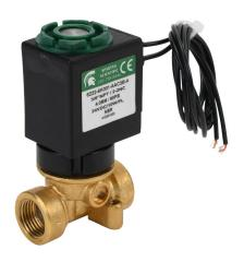
Spartan solenoid valve, 2-way, 2-position, N.C., low lead brass body, 3/8in female NPT inlet(s), 3/8in female NPT outlet(s), Cv=0.52, 90 psi maximum operating pressure, 24 VDC operating voltage, 18in 22 AWG pigtail.
