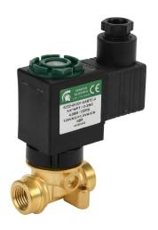
Spartan solenoid valve, 2-way, 2-position, N.C., low lead brass body, 1/4in female NPT inlet(s), 1/4in female NPT outlet(s), Cv=0.52, 125 psi maximum operating pressure, 120 VAC operating voltage, 18mm DIN style wiring plug.
