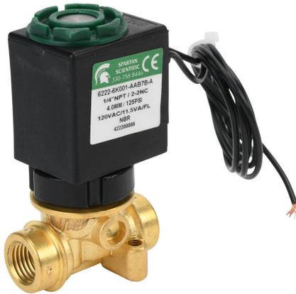
Spartan solenoid valve, 2-way, 2-position, N.C., low lead brass body, 1/4in female NPT inlet(s), 1/4in female NPT outlet(s), Cv=0.52, 125 psi maximum operating pressure, 120 VAC operating voltage, 18in 22 AWG pigtail.
