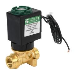
Spartan solenoid valve, 2-way, 2-position, N.C., low lead brass body, 1/4in female NPT inlet(s), 1/4in female NPT outlet(s), Cv=0.52, 125 psi maximum operating pressure, 120 VAC operating voltage, 18in 22 AWG pigtail.
