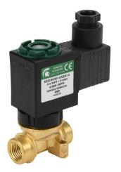
Spartan solenoid valve, 2-way, 2-position, N.C., low lead brass body, 1/4in female NPT inlet(s), 1/4in female NPT outlet(s), Cv=0.52, 90 psi maximum operating pressure, 24 VDC operating voltage, 18mm DIN style wiring plug.
