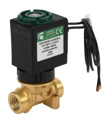
Spartan solenoid valve, 2-way, 2-position, N.C., low lead brass body, 1/4in female NPT inlet(s), 1/4in female NPT outlet(s), Cv=0.52, 90 psi maximum operating pressure, 24 VDC operating voltage, 18in 22 AWG pigtail.
