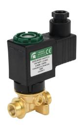
Spartan solenoid valve, 2-way, 2-position, N.C., low lead brass body, 1/8in female NPT inlet(s), 1/8in female NPT outlet(s), Cv=0.52, 125 psi maximum operating pressure, 120 VAC operating voltage, 18mm DIN style wiring plug.
