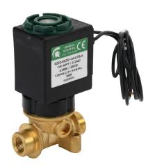
Spartan solenoid valve, 2-way, 2-position, N.C., low lead brass body, 1/8in female NPT inlet(s), 1/8in female NPT outlet(s), Cv=0.52, 125 psi maximum operating pressure, 120 VAC operating voltage, 18in 22 AWG pigtail.
