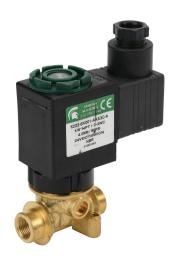
Spartan solenoid valve, 2-way, 2-position, N.C., low lead brass body, 1/8in female NPT inlet(s), 1/8in female NPT outlet(s), Cv=0.52, 90 psi maximum operating pressure, 24 VDC operating voltage, 18mm DIN style wiring plug.
