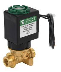
Spartan solenoid valve, 2-way, 2-position, N.C., low lead brass body, 1/8in female NPT inlet(s), 1/8in female NPT outlet(s), Cv=0.52, 90 psi maximum operating pressure, 24 VDC operating voltage, 18in 22 AWG pigtail.
