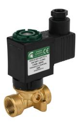
Spartan solenoid valve, 2-way, 2-position, N.C., low lead brass body, 3/8in female NPT inlet(s), 3/8in female NPT outlet(s), Cv=0.31, 270 psi maximum operating pressure, 120 VAC operating voltage, 18mm DIN style wiring plug.
