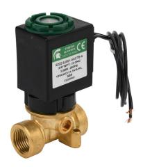
Spartan solenoid valve, 2-way, 2-position, N.C., low lead brass body, 3/8in female NPT inlet(s), 3/8in female NPT outlet(s), Cv=0.31, 270 psi maximum operating pressure, 120 VAC operating voltage, 18in 22 AWG pigtail.
