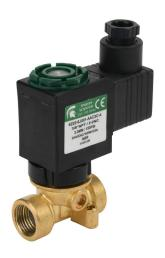
Spartan solenoid valve, 2-way, 2-position, N.C., low lead brass body, 3/8in female NPT inlet(s), 3/8in female NPT outlet(s), Cv=0.31, 150 psi maximum operating pressure, 24 VDC operating voltage, 18mm DIN style wiring plug.
