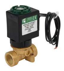
Spartan solenoid valve, 2-way, 2-position, N.C., low lead brass body, 3/8in female NPT inlet(s), 3/8in female NPT outlet(s), Cv=0.31, 150 psi maximum operating pressure, 24 VDC operating voltage, 18in 22 AWG pigtail.
