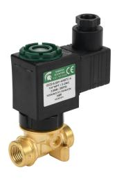
Spartan solenoid valve, 2-way, 2-position, N.C., low lead brass body, 1/4in female NPT inlet(s), 1/4in female NPT outlet(s), Cv=0.31, 270 psi maximum operating pressure, 120 VAC operating voltage, 18mm DIN style wiring plug.
