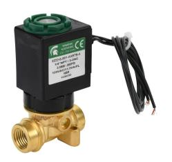
Spartan solenoid valve, 2-way, 2-position, N.C., low lead brass body, 1/4in female NPT inlet(s), 1/4in female NPT outlet(s), Cv=0.31, 270 psi maximum operating pressure, 120 VAC operating voltage, 18in 22 AWG pigtail.
