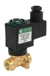
Spartan solenoid valve, 2-way, 2-position, N.C., low lead brass body, 1/4in female NPT inlet(s), 1/4in female NPT outlet(s), Cv=0.31, 150 psi maximum operating pressure, 24 VDC operating voltage, 18mm DIN style wiring plug.
