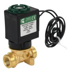
Spartan solenoid valve, 2-way, 2-position, N.C., low lead brass body, 1/4in female NPT inlet(s), 1/4in female NPT outlet(s), Cv=0.31, 150 psi maximum operating pressure, 24 VDC operating voltage, 18in 22 AWG pigtail.
