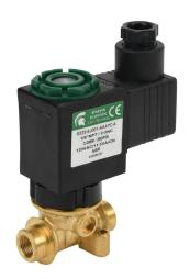
Spartan solenoid valve, 2-way, 2-position, N.C., low lead brass body, 1/8in female NPT inlet(s), 1/8in female NPT outlet(s), Cv=0.31, 270 psi maximum operating pressure, 120 VAC operating voltage, 18mm DIN style wiring plug.
