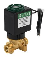
Spartan solenoid valve, 2-way, 2-position, N.C., low lead brass body, 1/8in female NPT inlet(s), 1/8in female NPT outlet(s), Cv=0.31, 270 psi maximum operating pressure, 120 VAC operating voltage, 18in 22 AWG pigtail.
