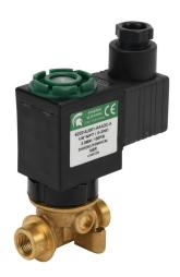
Spartan solenoid valve, 2-way, 2-position, N.C., low lead brass body, 1/8in female NPT inlet(s), 1/8in female NPT outlet(s), Cv=0.31, 150 psi maximum operating pressure, 24 VDC operating voltage, 18mm DIN style wiring plug.
