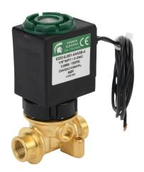
Spartan solenoid valve, 2-way, 2-position, N.C., low lead brass body, 1/8in female NPT inlet(s), 1/8in female NPT outlet(s), Cv=0.31, 150 psi maximum operating pressure, 24 VDC operating voltage, 18in 22 AWG pigtail.
