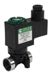
Spartan solenoid valve, 2-way, 2-position, N.C., glass-filled nylon body, 3/8in female NPT inlet(s), 3/8in female NPT outlet(s), Cv=0.72, 40 psi maximum operating pressure, 120 VAC operating voltage, 18mm DIN style wiring plug.
