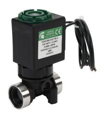
Spartan solenoid valve, 2-way, 2-position, N.C., glass-filled nylon body, 3/8in female NPT inlet(s), 3/8in female NPT outlet(s), Cv=0.72, 40 psi maximum operating pressure, 120 VAC operating voltage, 18in 22 AWG pigtail.
