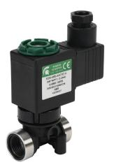
Spartan solenoid valve, 2-way, 2-position, N.C., glass-filled nylon body, 3/8in female NPT inlet(s), 3/8in female NPT outlet(s), Cv=0.72, 30 psi maximum operating pressure, 24 VDC operating voltage, 18mm DIN style wiring plug.
