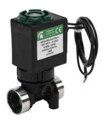
Spartan solenoid valve, 2-way, 2-position, N.C., glass-filled nylon body, 3/8in female NPT inlet(s), 3/8in female NPT outlet(s), Cv=0.72, 30 psi maximum operating pressure, 24 VDC operating voltage, 18in 22 AWG pigtail.
