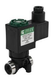
Spartan solenoid valve, 2-way, 2-position, N.C., glass-filled nylon body, 1/4in female NPT inlet(s), 1/4in female NPT outlet(s), Cv=0.61, 50 psi maximum operating pressure, 120 VAC operating voltage, 18mm DIN style wiring plug.
