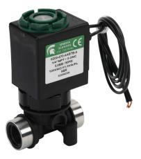
Spartan solenoid valve, 2-way, 2-position, N.C., glass-filled nylon body, 1/4in female NPT inlet(s), 1/4in female NPT outlet(s), Cv=0.61, 50 psi maximum operating pressure, 120 VAC operating voltage, 18in 22 AWG pigtail.
