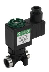
Spartan solenoid valve, 2-way, 2-position, N.C., glass-filled nylon body, 1/4in female NPT inlet(s), 1/4in female NPT outlet(s), Cv=0.61, 50 psi maximum operating pressure, 24 VDC operating voltage, 18mm DIN style wiring plug.
