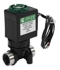
Spartan solenoid valve, 2-way, 2-position, N.C., glass-filled nylon body, 1/4in female NPT inlet(s), 1/4in female NPT outlet(s), Cv=0.61, 50 psi maximum operating pressure, 24 VDC operating voltage, 18in 22 AWG pigtail.
