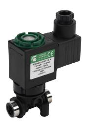
Spartan solenoid valve, 2-way, 2-position, N.C., glass-filled nylon body, 1/8in female NPT inlet(s), 1/8in female NPT outlet(s), Cv=0.52, 75 psi maximum operating pressure, 120 VAC operating voltage, 18mm DIN style wiring plug.
