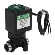
Spartan solenoid valve, 2-way, 2-position, N.C., glass-filled nylon body, 1/8in female NPT inlet(s), 1/8in female NPT outlet(s), Cv=0.52, vacuum minimum operating pressure, 120 VAC operating voltage, 18in 22 AWG pigtail.
