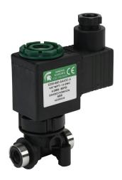
Spartan solenoid valve, 2-way, 2-position, N.C., glass-filled nylon body, 1/8in female NPT inlet(s), 1/8in female NPT outlet(s), Cv=0.52, 80 psi maximum operating pressure, 24 VDC operating voltage, 18mm DIN style wiring plug.
