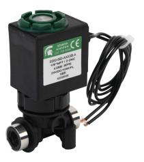
Spartan solenoid valve, 2-way, 2-position, N.C., glass-filled nylon body, 1/8in female NPT inlet(s), 1/8in female NPT outlet(s), Cv=0.52, 80 psi maximum operating pressure, 24 VDC operating voltage, 18in 22 AWG pigtail.
