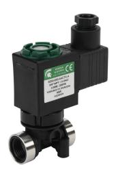
Spartan solenoid valve, 2-way, 2-position, N.C., glass-filled nylon body, 3/8in female NPT inlet(s), 3/8in female NPT outlet(s), Cv=0.31, 250 psi maximum operating pressure, 120 VAC operating voltage, 18mm DIN style wiring plug.
