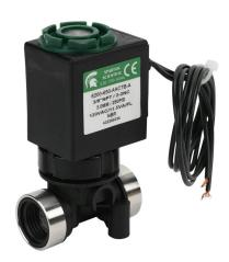
Spartan solenoid valve, 2-way, 2-position, N.C., glass-filled nylon body, 3/8in female NPT inlet(s), 3/8in female NPT outlet(s), Cv=0.31, 250 psi maximum operating pressure, 120 VAC operating voltage, 18in 22 AWG pigtail.
