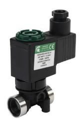
Spartan solenoid valve, 2-way, 2-position, N.C., glass-filled nylon body, 3/8in female NPT inlet(s), 3/8in female NPT outlet(s), Cv=0.31, 150 psi maximum operating pressure, 24 VDC operating voltage, 18mm DIN style wiring plug.
