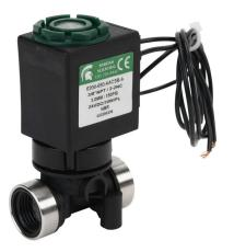
Spartan solenoid valve, 2-way, 2-position, N.C., glass-filled nylon body, 3/8in female NPT inlet(s), 3/8in female NPT outlet(s), Cv=0.31, 150 psi maximum operating pressure, 24 VDC operating voltage, 18in 22 AWG pigtail.
