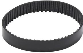
SureMotion timing belt, 0.08in MXL pitch, 1/4in wide, 61 tooth, 4.9in pitch length (circumference), polyurethane, polyester reinforced. Package of 3.
