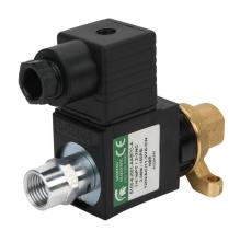
Spartan solenoid valve, 2-way, 2-position, N.C., low lead brass body, 1/4in female NPT inlet(s), 1/4in female NPT outlet(s), Cv=0.31, 150 psi maximum operating pressure, 120 VAC operating voltage, 18mm DIN style wiring plug.
