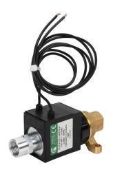
Spartan solenoid valve, 2-way, 2-position, N.C., low lead brass body, 1/4in female NPT inlet(s), 1/4in female NPT outlet(s), Cv=0.31, 150 psi maximum operating pressure, 120 VAC operating voltage, 18in 22 AWG pigtail.
