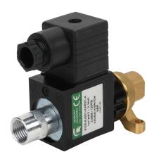
Spartan solenoid valve, 2-way, 2-position, N.C., low lead brass body, 1/4in female NPT inlet(s), 1/4in female NPT outlet(s), Cv=0.31, 120 psi maximum operating pressure, 24 VDC operating voltage, 18mm DIN style wiring plug.
