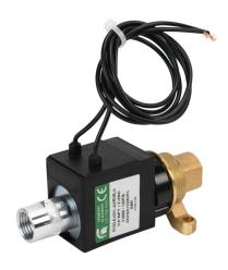
Spartan solenoid valve, 2-way, 2-position, N.C., low lead brass body, 1/4in female NPT inlet(s), 1/4in female NPT outlet(s), Cv=0.31, 120 psi maximum operating pressure, 24 VDC operating voltage, 18in 22 AWG pigtail.
