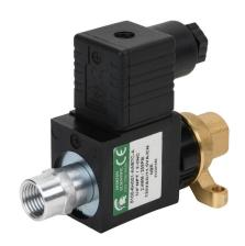
Spartan solenoid valve, 2-way, 2-position, N.C., low lead brass body, 1/4in female NPT inlet(s), 1/4in female NPT outlet(s), Cv=0.24, 255 psi maximum operating pressure, 120 VAC operating voltage, 18mm DIN style wiring plug.
