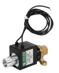
Spartan solenoid valve, 2-way, 2-position, N.C., low lead brass body, 1/4in female NPT inlet(s), 1/4in female NPT outlet(s), Cv=0.24, 255 psi maximum operating pressure, 120 VAC operating voltage, 18in 22 AWG pigtail.
